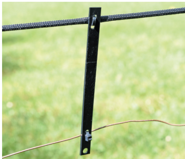
Figure 13 — Sturdy \frac{3}{8} -inch UV-resistant dacron/polyester rope supports the #18 AWG solid antenna wire. The wire is quite stiff, and it takes some experimentation to get it to look like the photo at www.hybriddx.com .
